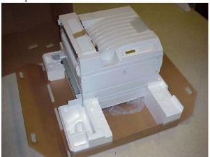
**9.** Box the Print Cartridge and place box onto the foam blocks.
