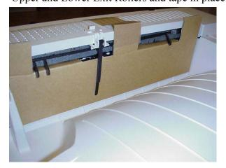
**2.** Remove MBF Assembly from Printer by pulling Up and Outward.
