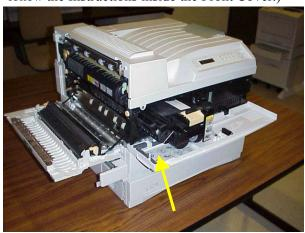
**5.** Insert the Cardboard Support between the Upper and Lower Exit Rollers and tape in place.
