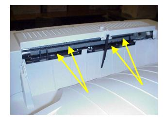
**6.** Tape shipping pad to Printer as shown.
